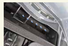
Holes on the muffler disperse exhaust cooling it
