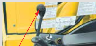
● Travel speed select switch The travel speed select switch is placed on the dozer lever and it allows selecting the travel speed.
