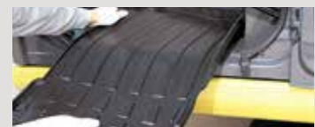
• Detachable two-piece floor mat with handles for easy removal. A floor drain located under floor mat is easily removed without tools for cleaning
