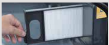
• Internal and external air conditioner filters can be easily removed without tools for cleaning
