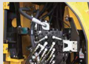
• Easy access to main control valves (Front)
