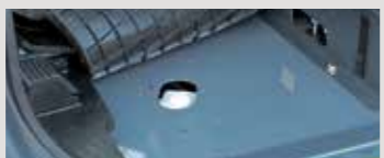
• Washer fluid tank located under the cab floor mat.
