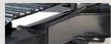
• Special crawler frame designed is easily cleaned of mud
