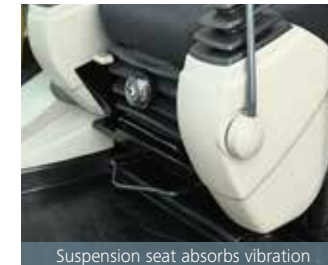
Suspension seat absorbs vibration
