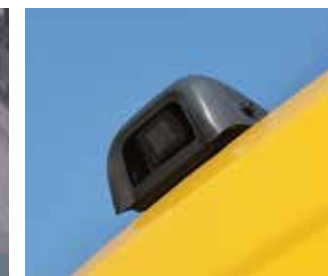
Standard rear-view camera eases safety checks behind the machine. Color video displays on cab monitor.
