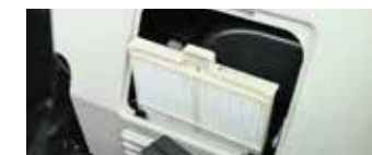
Air conditioner filter can be easily removed without tools for cleaning. One for outside air and one for inside air.
