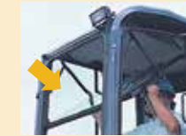
Front window features gas damper cylinders for smooth and easy opening.
