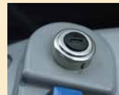
Easy-access, easy-turn ignition with rubber boots for protection against moisture and freezing
