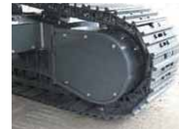
Reinforced guard for travel motor Thick steel plate used to ensure strength and protect drive motors.
