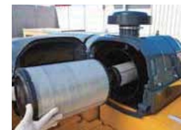
Air cleaner (double element) The double filter system provides clean and filtered air for the engine.
