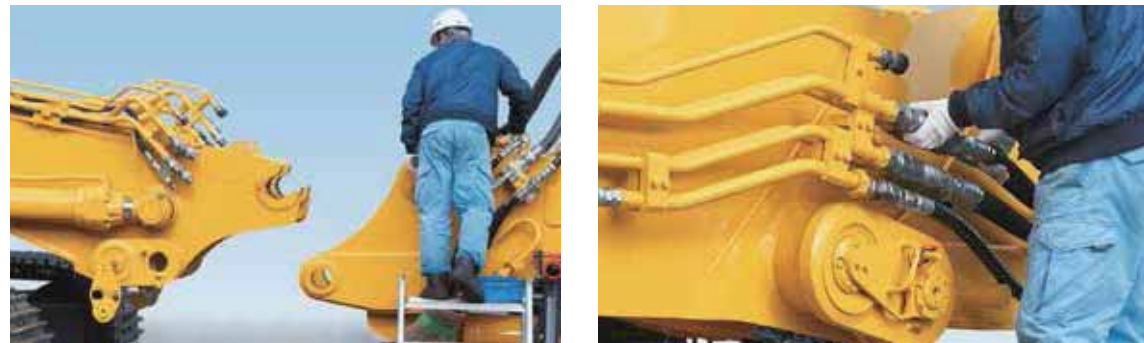
Piping connection: Hydraulic quick coupler system on the side of the boom.
