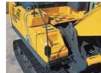
Maintenance space Large open space on top of machine to easily service and inspect engine.
