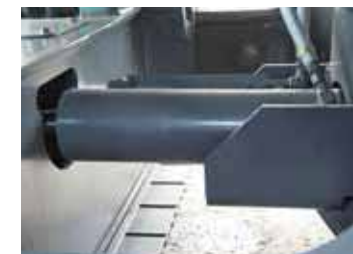
Crawler extension/retraction mechanism guard Hydraulic cylinders are protected from debris. [on SK400DLC and SK550DLC]
