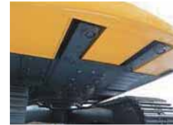
Upper frame belly guards The 0.24"(6mm) thick reinforced cover protects the inner devices & engine unit.
