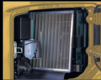
Ground level maintenance iNDr filter
