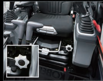
Adjustable height pilot valves Operator can adjust height of attachment control levers (Only for optional Air Ride Suspension Seat.)
