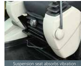
Suspension seat absorbs vibration
