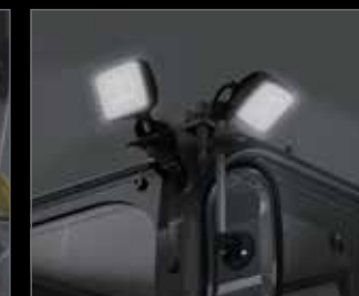
Forward and Left-Facing LED Light (Cab)
