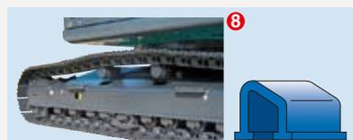
8 Special crawler frame design is easily cleaned of mud.
