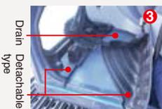
3 Detachable two-piece floor mat with handles for easy removal. A floor drain is located under the mat.
