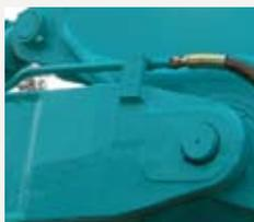
Integrated cast steel boom top
