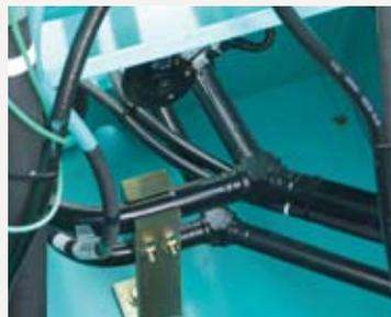
Rigorous inspections for pressure loss are performed on all components of the hydraulic piping, from the first spool of the control valve to the connectors. This regimen, combined with the use of a new, high-efficiency pump, cuts energy loss to a minimum.
