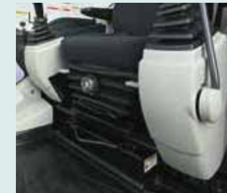
Seat suspension absorbs vibration
