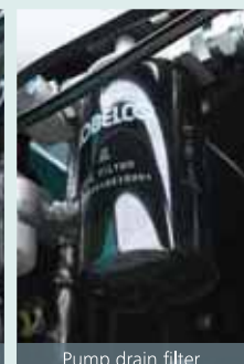
Pump drain filter
