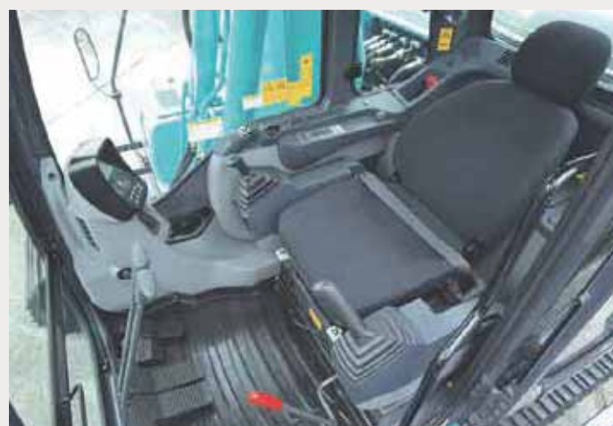
● Seat can be reclined to horizontal position
