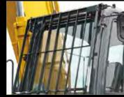
Wire Mesh or Vertical Bar **Front Cab Guard (optional)**
