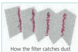
\* “60-mesh” means that there are 60 holes formed by horizontal and vertical wires in every square inch of filter.
