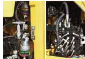
Fuel water separator/Fuel filter/Control valve
