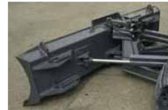
The 6-way dozer blade has Power, Angle and Tilt capability (PAT) operated from the cab. With a single control lever, the blade can be angled 25 degrees to the left or right for dispensing earth and materials away from the operator's path. The blade also tilts up on the left and right sides by 1' 6" {455 mm} for slope grading, culverts and ditches.
