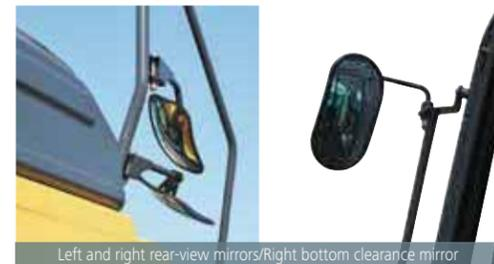
Left and right rear-view mirrors/Right bottom clearance mirror
