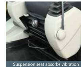
Suspension seat absorbs vibration
