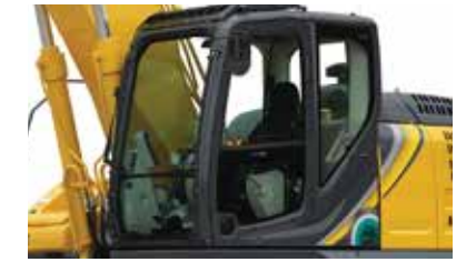
Mounting brackets for vandalism guards are standard equipment (contact your KOBELCO dealer to fit vandalism or front rock guards).
