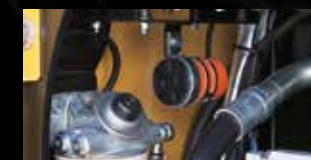
Travel alarm The alarm cautions workers in the area that the machine is traveling.
