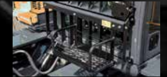
Work boot tray This space was added to hold work boots in order to keep the floor of the cab clean.
