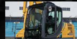
Front guard (wire mesh guard) Front windows are protected by a wire mesh guard to prevent damage and provide additional safety for the operator.
