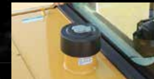
Dust-proof fuel tank cap The fuel cap is lined with rubber to prevent dust from contaminating the fuel tank.
