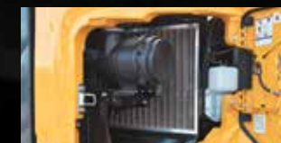
INDr filter [only SK140SRD] The corrugated filter design prevents clogging to reduce maintenance and assists to reduce noise.
