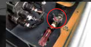
Remote fuel drain valve [only SK140SRD] Allows for easy fuel draining if required.
