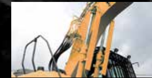
Boom cylinder guard A steel-plate guard is equipped to protect the boom cylinder rod from damage.
