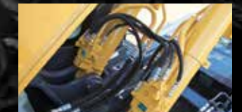
Boom & arm holding valves Standard - to prevent boom or arm from falling if hose is damaged.
