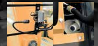
Public address system Operator is able to alert ground workers without taking their hands off the machine controls.
