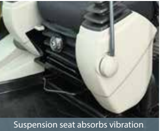
Suspension seat absorbs vibration
