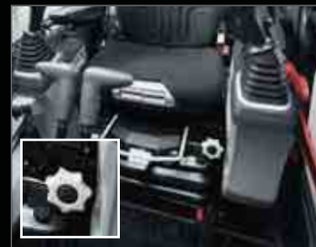
Adjustable height pilot valves Operator can adjust height of attachment control levers
