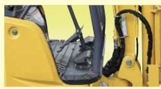
Pass-through operating station allows getting on and off from either side.
