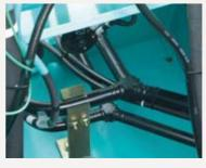
Rigorous inspections for pressure loss are performed on all components of the hydraulic piping, from the spool of the control valve to the connectors. This regimen, combined with the use of a new, high-efficiency pump, cuts energy loss to a minimum.
