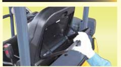
The operator's manual storage is located on the back side of the operator's seat.
