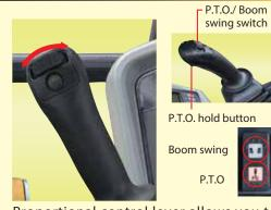
Proportional control lever allows you to control boom swing operation and the attachment easily.
